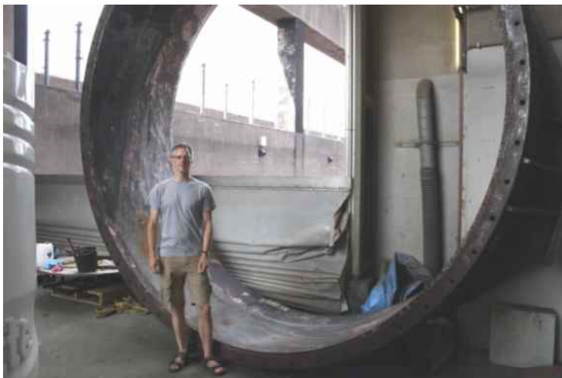
Figure 5.4. Impeller housing from one of the pumps at IJmuiden.
