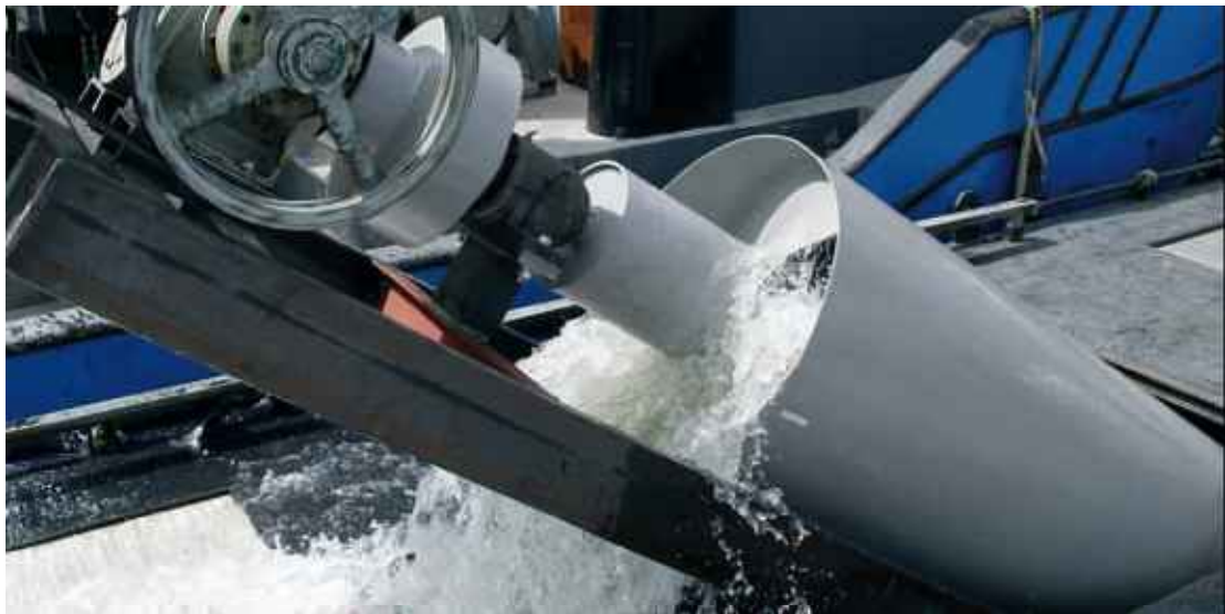
Figure 5.9. Top end of an Archimedes Screw pump with a fixed tube or shroud throughout its length. Photograph courtesy of Fish Flow Innovations.
