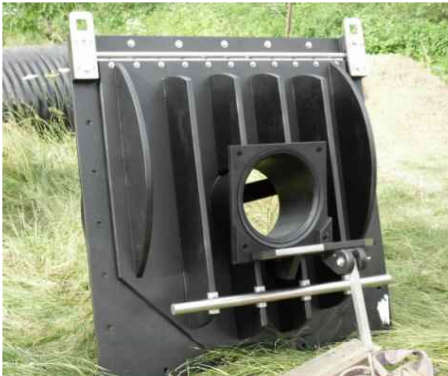
Figure 3.19. An ACE HDPE tidal flap fitted with a 300 mm internal diameter cat flap. The cat flap door is open, and is operated by a float which would be attached to the hinged metal rod attached to the front edge of the flap. Photograph courtesy of ACE.
