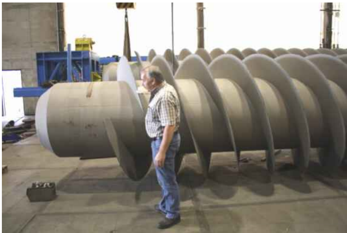
Figure 5.6. Archimedes screw runners at the Landustrie factory for refurbishment. These are about 1.8 m diameter, but they have been made up to 5 m in diameter and 25 m in length.
