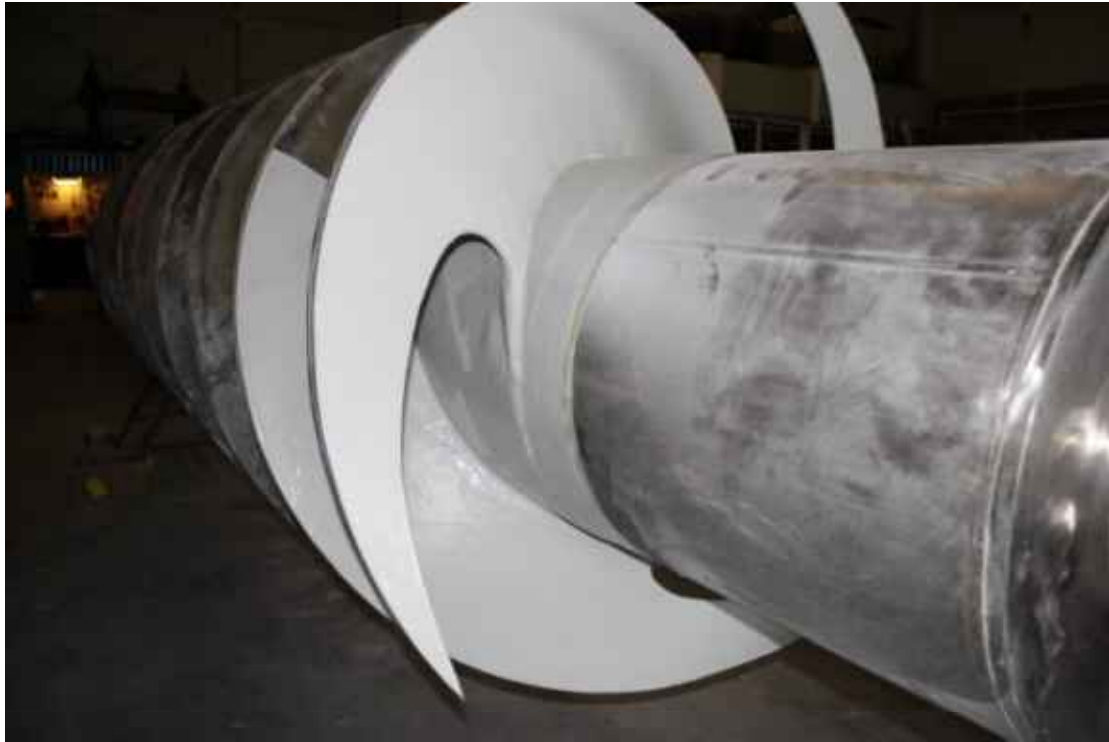
Figure 5.8. Lower end of a Fish Flow Innovations Archimedes screw pump under construction. The shape of the blade leading edge minimises collision risk and damage. The whole screw will be fitted within a rotating tube so that blade-edge gaps are eliminated. The diameter is 1.4 m, and the pumping capacity is 0.26 m 3 /sec at 38 rpm over a head of 1.24 m.
