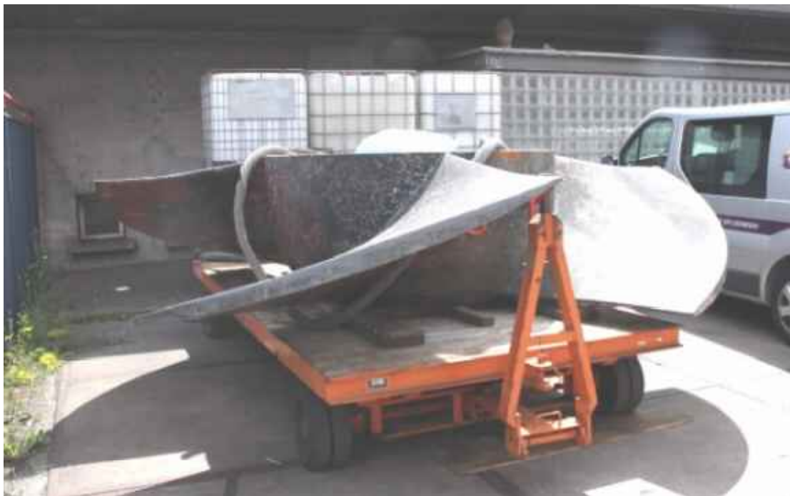
Figure 5.3. Pump impeller from one of the eight axial-flow pumps at IJmuiden, removed for maintenance.
